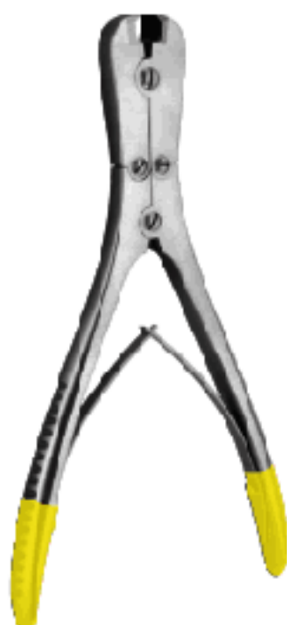
Vital Wire Cutter F9-795 18cm 7" for hard wires up to 1.7mm, for soft wires up to 2mm
