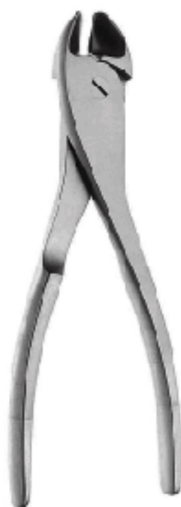
Side Cutter F9-708 18.5cm 7 1/4" Welded carbide jaws max capacity: 1.6mm 062"
