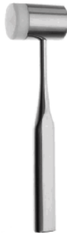
Combination Mallet F9-041 19.5cm 7 5/8" Solid. Head diameter 32.0mm, Weight: 12 cz 340 grams. Head weight: 8 cz 227 grams
